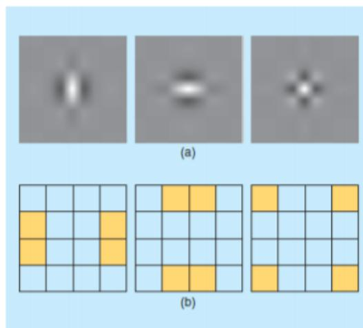
**Fig 3** Typical wavelets associated with the 2-D separable DWT
