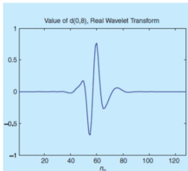
**Fig 1** Real DWT producing large and small wavelet coefficients
